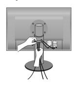
**3.** Please put the power cord and the signal cable in the cable holder 2. While pressing the bottom of cable holder 2 with one hand, pull the top of it with the other hand as shown in the picture.
